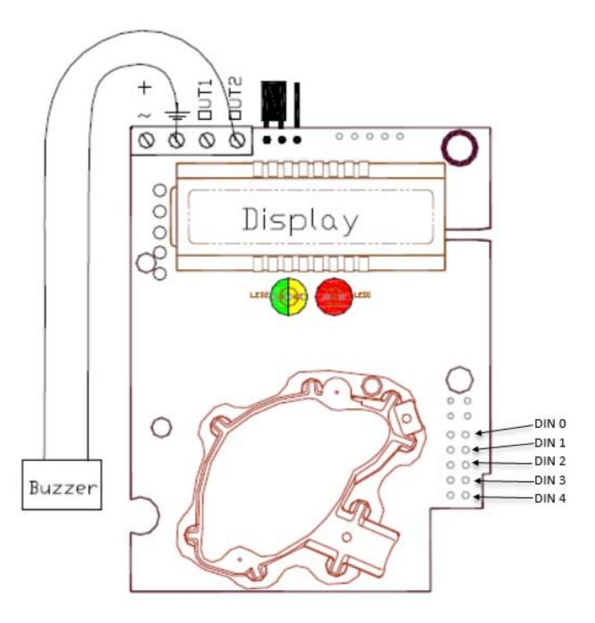
Jumper Din2 for 0 ppm CO2 calibration or Din3 for 400 ppm CO2 for a minimum of 8 seconds
