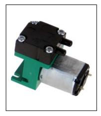
In a dry running diaphragm pump, a flexible diaphragm in the pump head moves up and down through the action of an eccentric on the motor shaft. On the down stroke, air is drawn into the pump chamber and expelled on the upstroke. One-way flap valves mounted within the pump head control the direction of flow of air. Equally suitable for use as a vacuum pump or compressor, these micro gas pumps are characterized by low noise, high efficiency and gas tightness.
