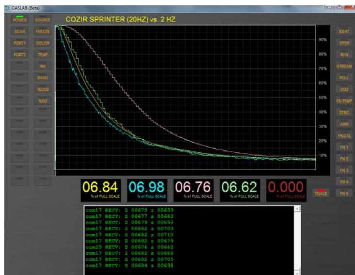
Figure 2 shows the response when ambient air is flowed into the unit. Note the cyan SprintIR instantaneous fall-off.
