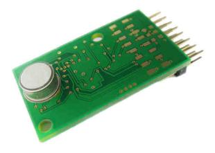
During the first 6 hours of continuous operation (burn-in) the module will display 350ppm, 2.5VDC, 50%PWM. The successful burn-in is saved to the EEPROM, the run-in time after restart is 15min.
