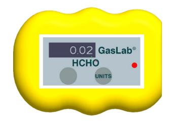
The GasLab SAN-103 is a wearable, personal safety meter designed to monitor formaldehyde concentrations (CH2O or H-CHO) in real time. Formaldehyde is a colorless, poisonous, highly water-soluble gas with an obnoxious odor. At high levels over time, it is a known carcinogen.
