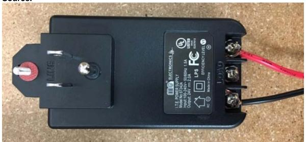
The +24VDC Power Adapter will power the RAD-0102-6 and the Safety Shut-Off Valve.
